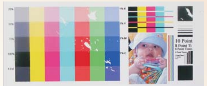
Ink jet pigment print on microporous paper, after immersion in water and blotter-drying. Flaking of image can be seen. Image shows no dye bleeding.
