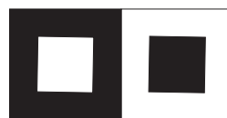
Figure 28. Knife-edge target for resolution measurement. Can also be used for flare measurement.
