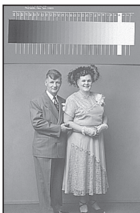
Figure 14. Calibrated gray-scale test targets serve as a link back to the reality of the original document or photograph.
